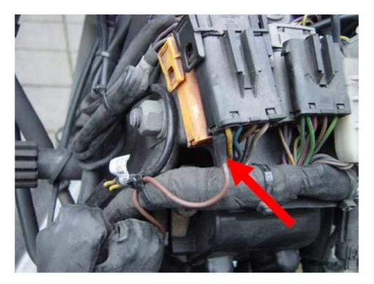
We're now done with fitting the wires. Tie the wiring solder points back together again and insulate them with some self-vulcanising tape.
