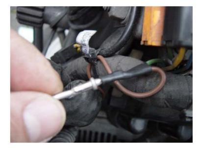
Fit the connector pin back into the connector block and refit the handlebar switch connector block.
