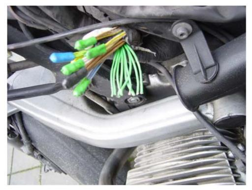
Now we need to find out which of these wires are connected to the ABS system and which are not.
