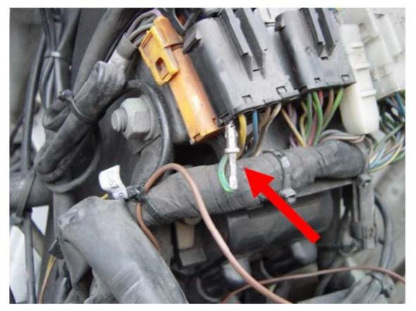
Removing this connector is best done with a special tool. If you manage to remove this connector, solder the brown wire from the bunch of 3 green wires on to the connector pin and insulate it using a piece of heat shrink.
