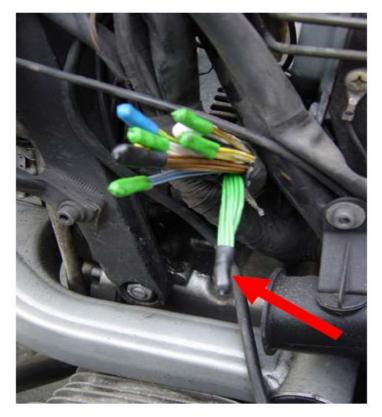
Cut the black insulating cap open and cut off the cap connecting the wires together. This will leave you with a bunch of 9 loose wires.
