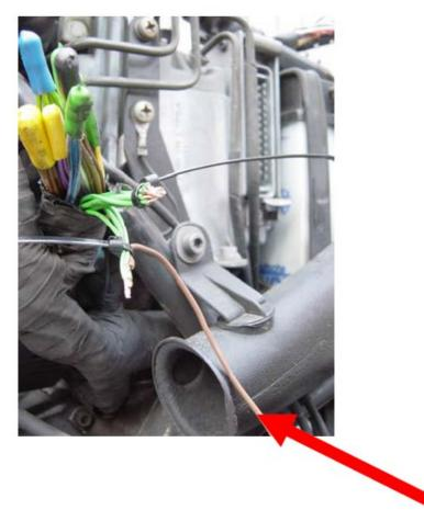
Solder or crimp the ends of the two bunches, and insulate them with heat shrink tape or similar.
