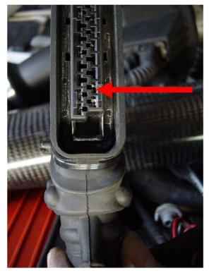
Attach one end of a multimeter to this connector pin, and find the other end of this wire in the bunch of 9 loose wires. Once you've found the corresponding wire, mark it so you can recognise it (e.g. attach a label or a piece of tape).
