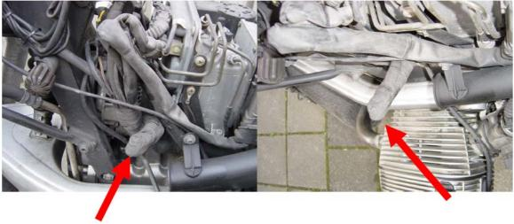
This solder point is at the back of the wiring harness. Remove the cotton tape which is wrapped around the solder point. This will reveal several different wiring "nodes" or bundles.
