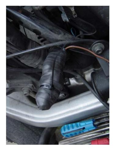
Push the solder point bunch back in place and tie-wrap everything in place. Refit the ABS control unit connector and the ABS relay. Reconnect the battery and set the time display. Replace the tank and the front and rear seats, and you're done!
