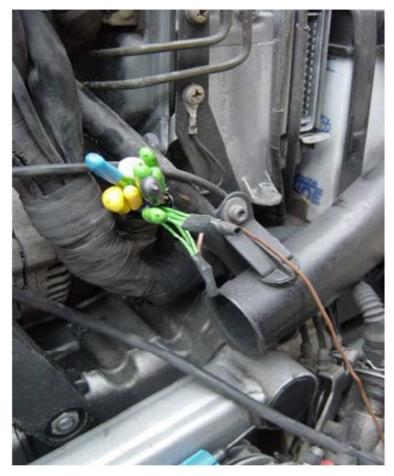
Route the brown wire (or whatever colour you used) up towards the connector block on top of the frame, just below the tank.
