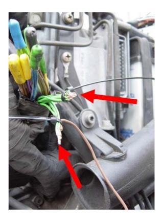
Now, add a wire of the same gauge as the green wires to bunch of 3 green ABS wires. (In the picture, the brown wire).
